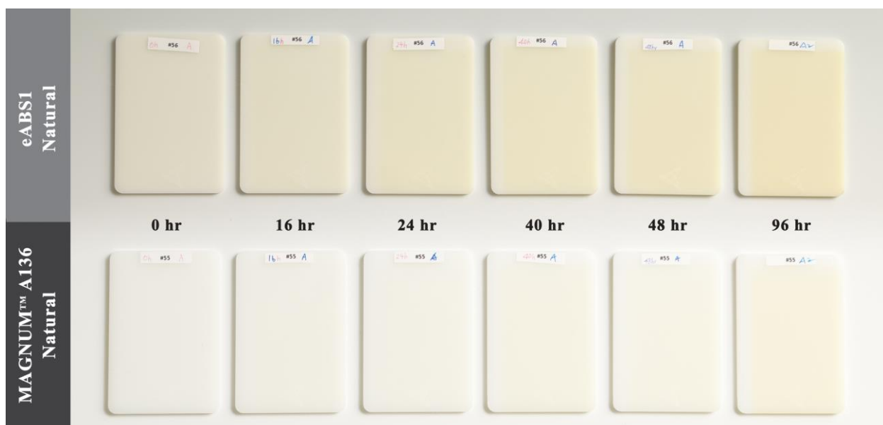
Figure 3: Photographic color shift of natural ABS resins with exposure time in QUV-A test
